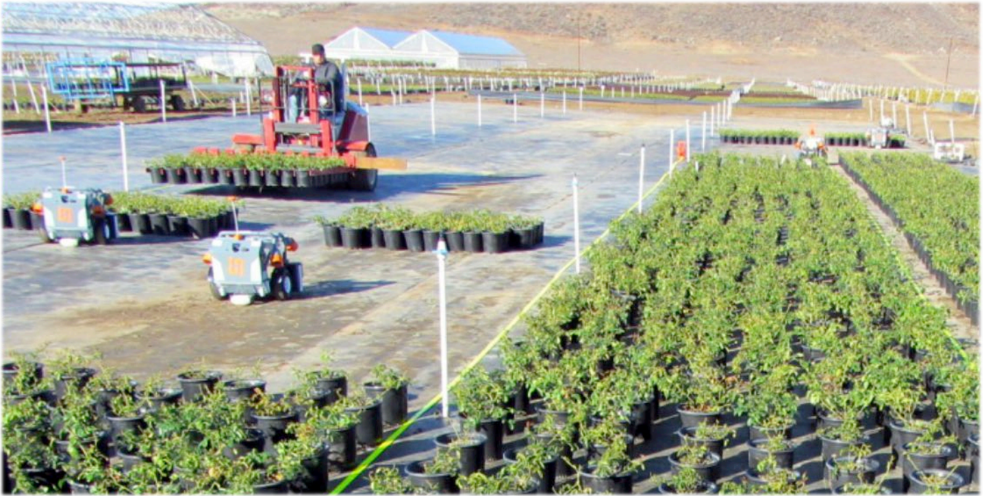
Robot Wrangler Miguel operating bedding forks while simultaneously supervising four Harvest Automation HV-100s.
